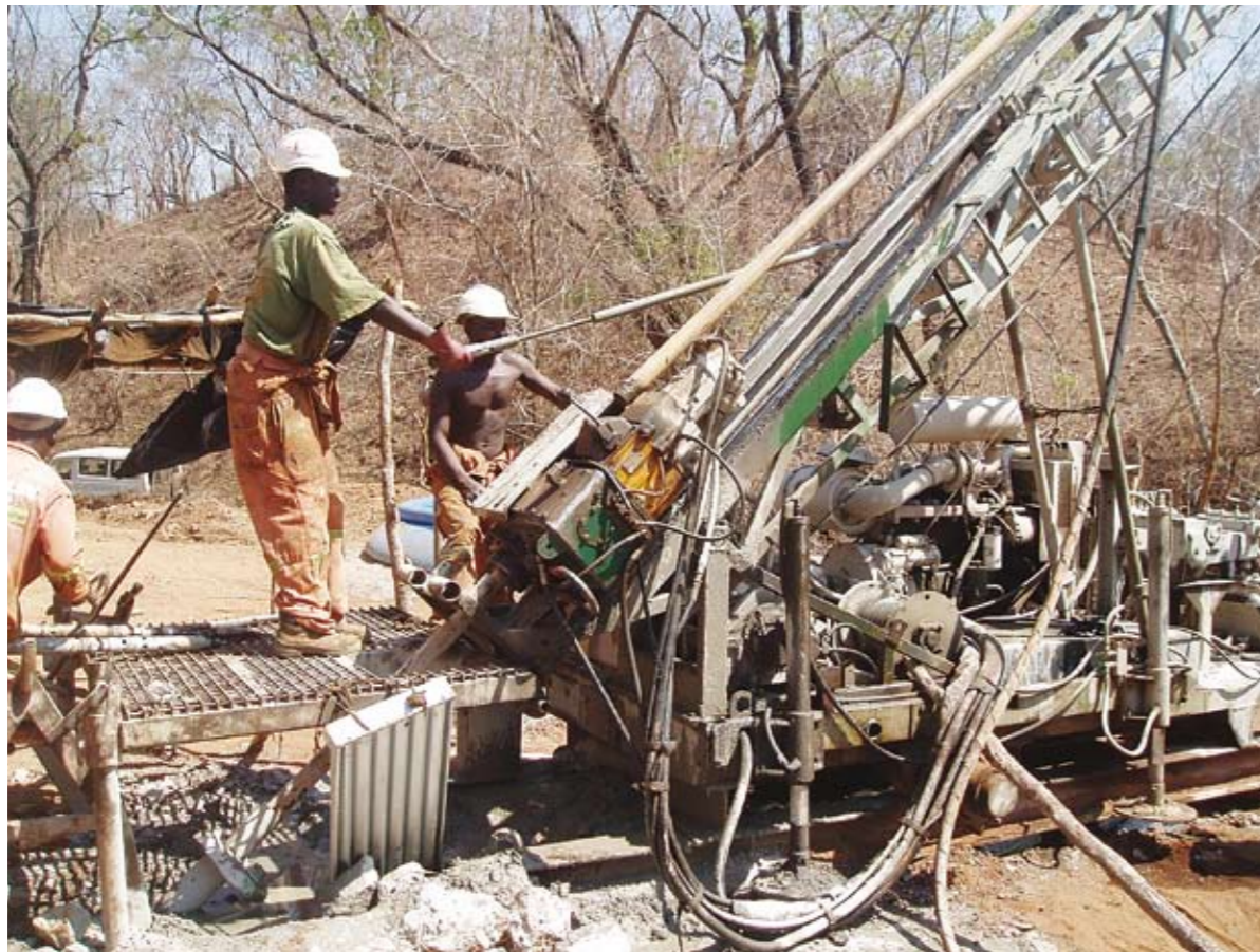
A diamond drill rig working on Zambezi's Chakwenga gold project in southern Zambia.
