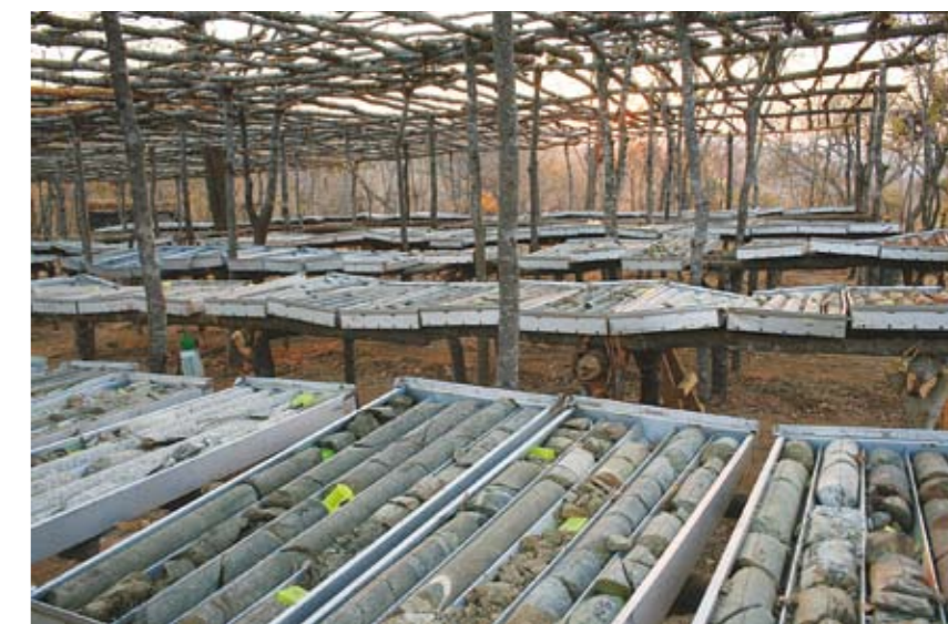
Drill core samples at the Cheowa site. Drilling at Cheowa in 2007 amounted to almost 40 000 m.
